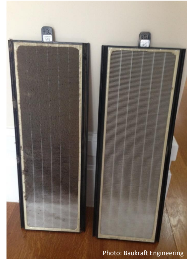
Left: outdoor air filter Right: exhaust air filter
