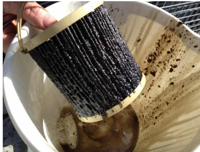
Clogged car filter
