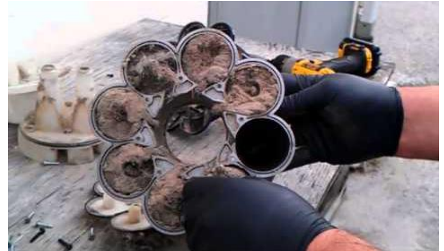
Clogged vacuum filter
