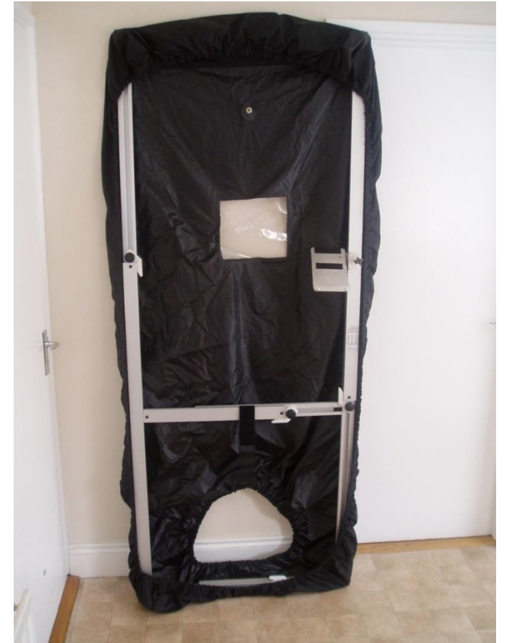
Canvas draped over frame, with circular hole at bottom to accommodate the fan
