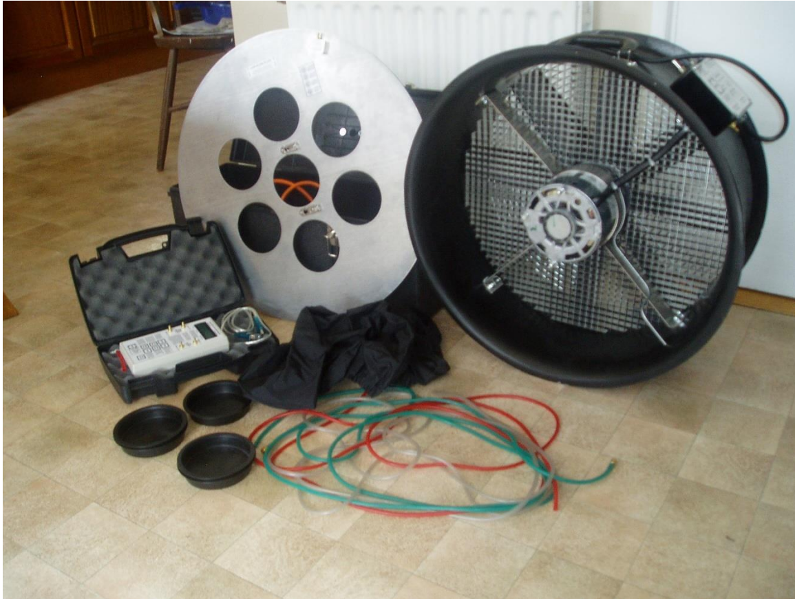
Fan used to create the pressure difference between inside and outside the building
